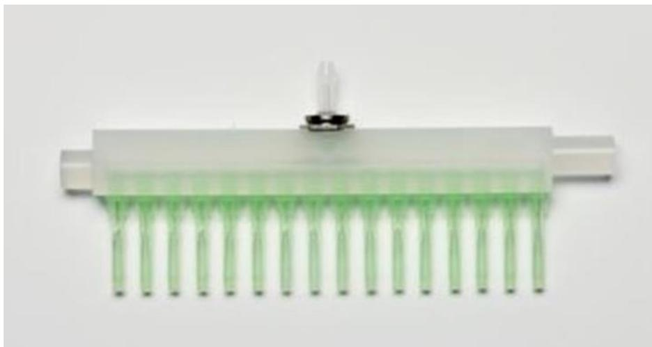
**Illustration 8.5:** 16 tip manifold with 0.015 ID tips for a 10 ml syringe
