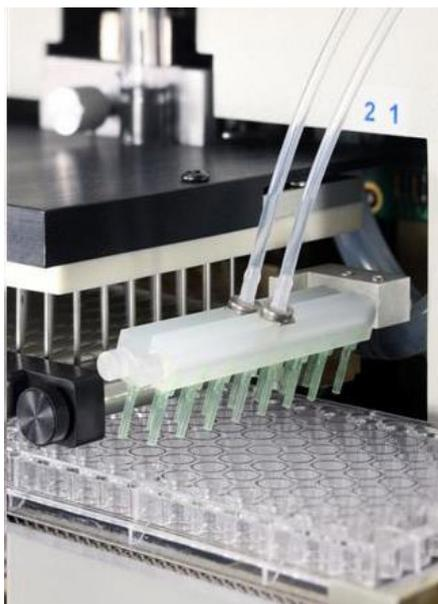
**Illustration 4.4:** Correct Manifold Positioning for the Dispense Module
