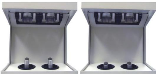
**Illustration 8.8:** The piston drive rods before install syringe mode (left) and during install syringe mode (right)
